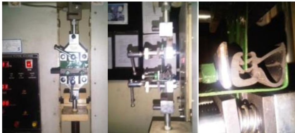
Insertion & Exertion Force Digital Testing
