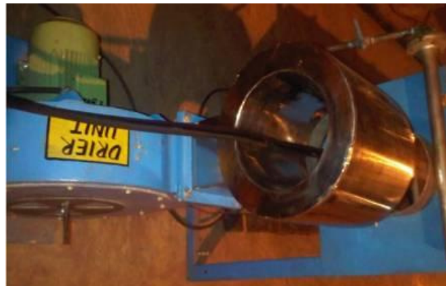
Rubber Profiles Dried Automatically online after Cooling & Cleaning in water
