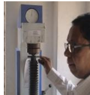
Hardness Tester Machine (Rockwell & BHN) & Eye Piece
