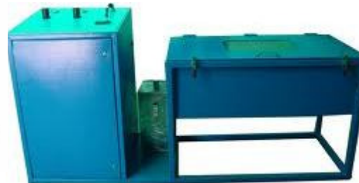
High Pressure Hose Hydro pneumatic Burst Pressure measuring Test Facility
