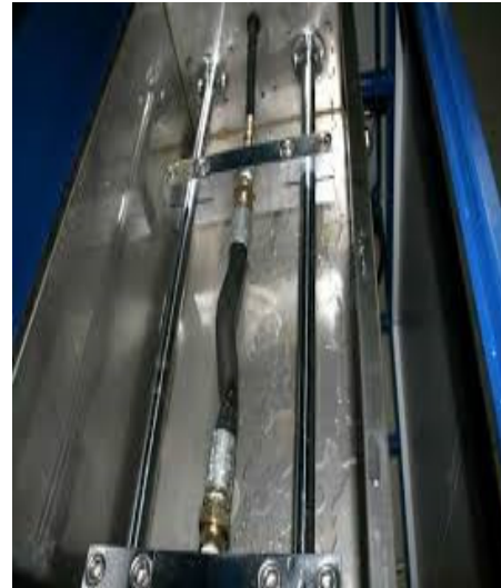
High Pressure Hose Hydro pneumatic Burst Pressure measuring Test Facility
