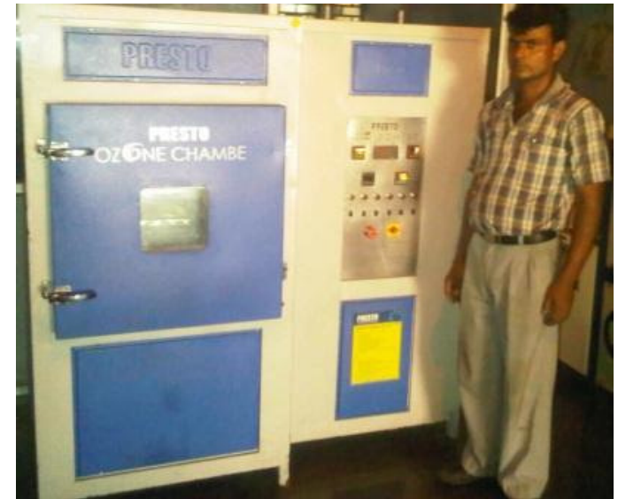
Ozone Testing Chamber: Static & Dynamic Testing
