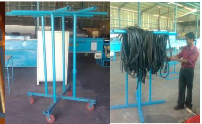
Special Hangers for Hanging Rubber Profiles while in Production to avoid any scratch or cut.
