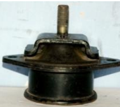
Hydro Mount with Rubber Piston-Cylinder for better Vibration absorption in cab
